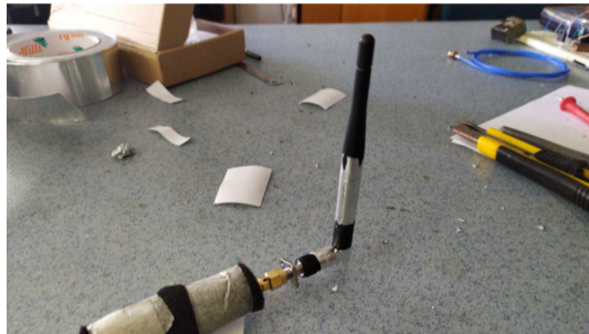
Monopole antenna tuning with aluminum tape
